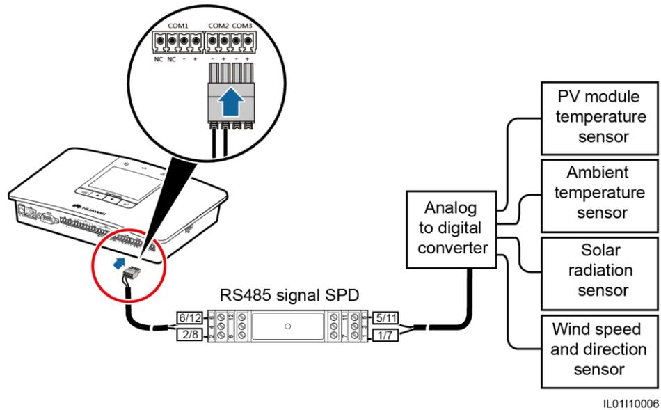
**Step 1** Prepare a cable with an appropriate length, strip a proper part of the insulation layer from one end, and connect the end to the port on the analog-to-digital converter.
