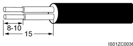
**Step 3** Insert the bare core wires into the surge port of the RS485 signal SPD, as shown by (1) in [Figure 4-25](#).
